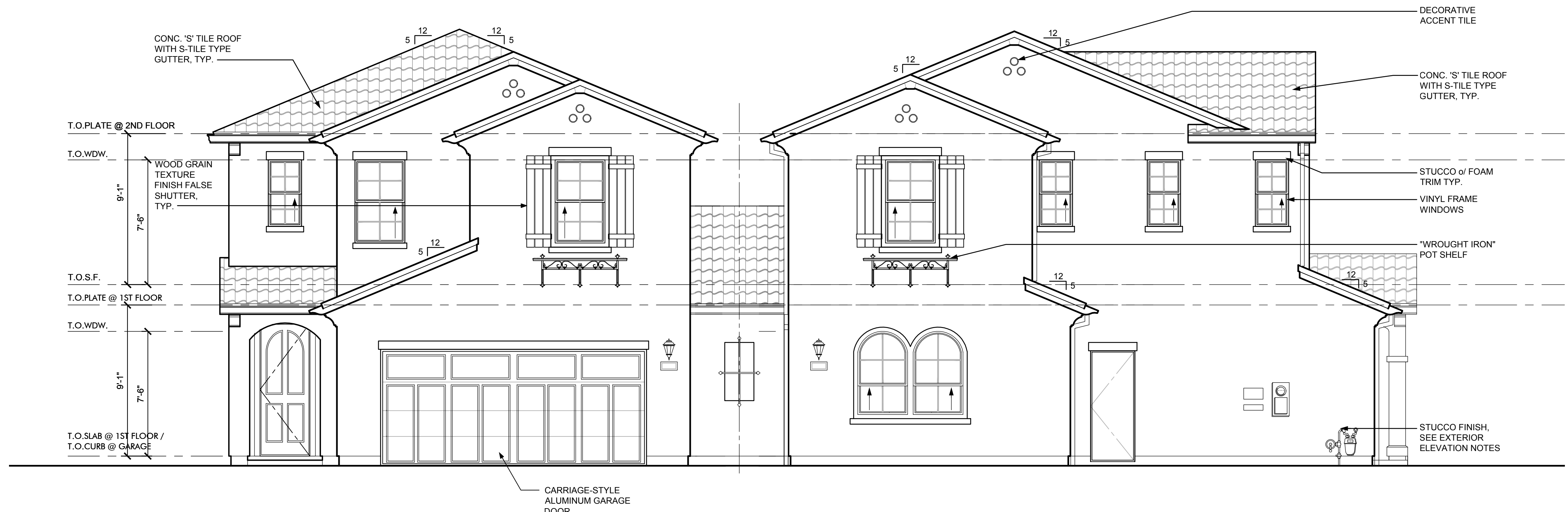
PLAN 1X FRONT ELEVATION B, SPANISH SCALE: 1/4" = 1'-0" PLAN 2X FRONT ELEVATION B, SPANISH SCALE: 1/4" = 1'-0" BUILDING 1X/2X FRONT ELEVATION B, SPANISH
