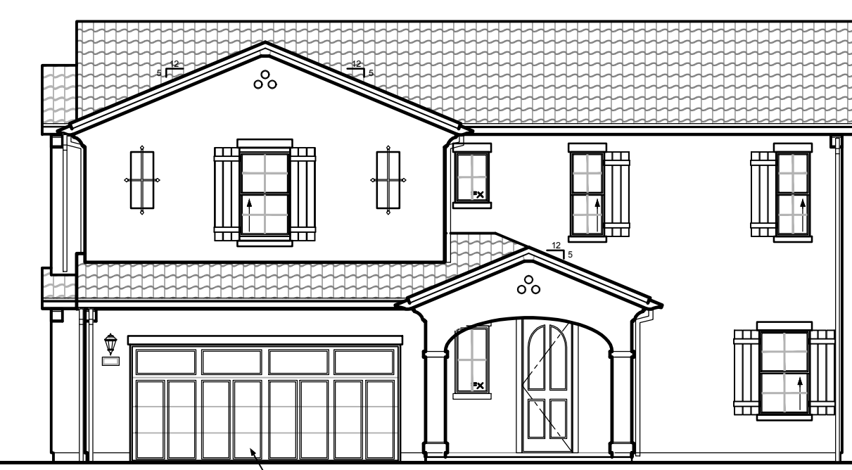
PLAN 2X RIGHT SIDE ELEVATION B, SPANISH SCALE: 1/4" = 1'-0" BUILDING 1X/2X RIGHT SIDE ELEVATION B, SPANISH
