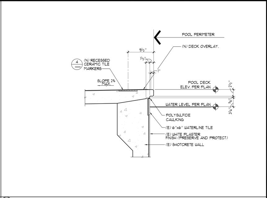
**3 EXISTING/NEW DECK AT BOND BEAM DETAIL** 1/2" = 1'-0"
