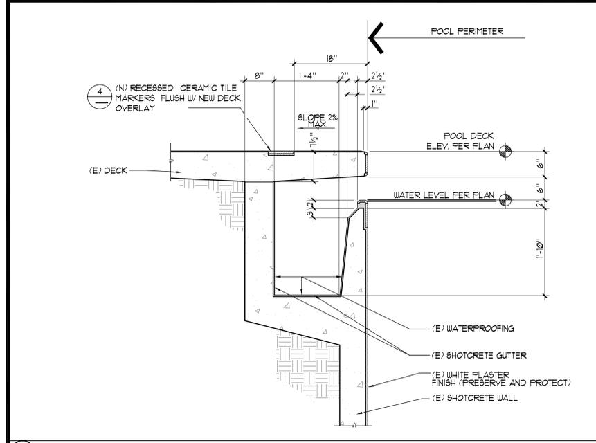
**1 EXISTING/NEW GUTTER DETAIL** 1" = 1'-0"
